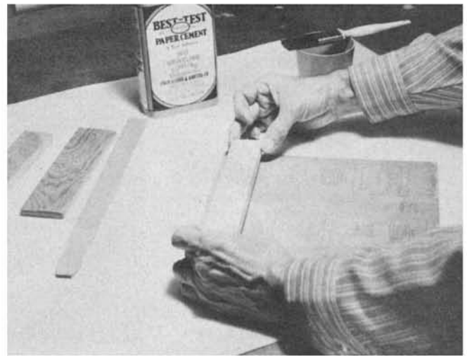
Start out by coating the back of the grit paper. We used Best Test Rubber Cement which is available at most art supply stores. Covering the work table with wax paper keeps the whole job neat.
