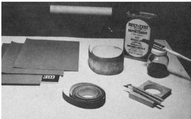
Basic materials for making sanding blocks include various grades of grit paper in sheets or strips, rubber base adhesive, brush, knives and cleaner. FLYING MODELS
