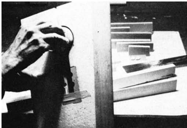
Use the cup to sand clean wheel wells with both the sides and bottom smooth enough to finish with a coat of epoxy resin. No need for balsa. FLYING MODELS
