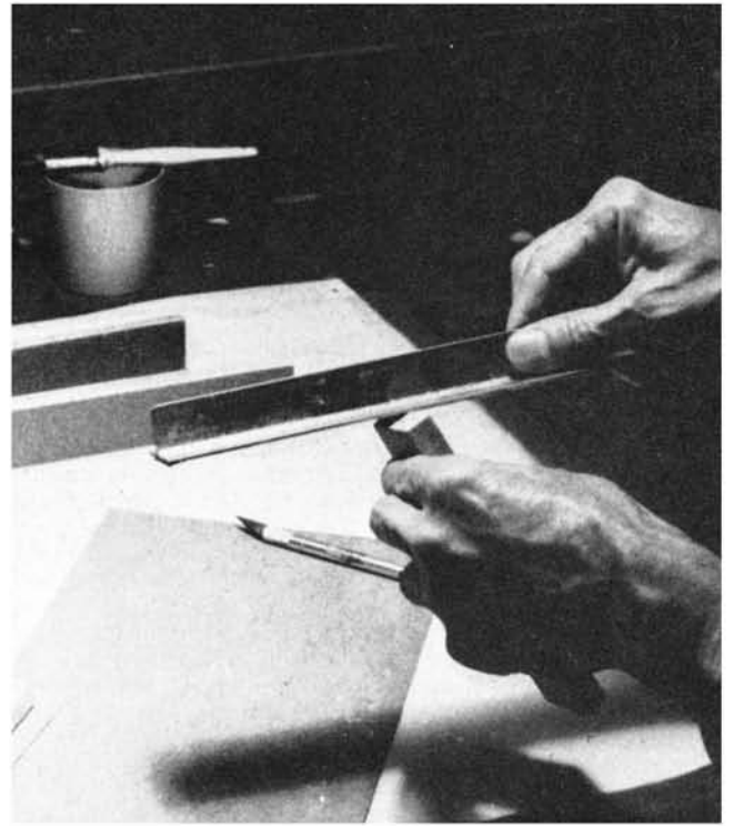
For fine trimming of the excess grit paper around one of your sanding blocks, use another sanding block. Trim across the grit as shown.
