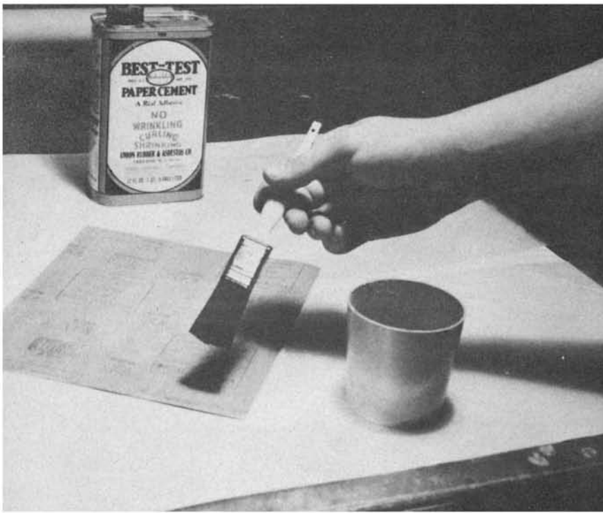
Start out by coating the back of the grit paper. We used Best Test Rubber Cement which is available at most art supply stores. Covering the work table with wax paper keeps the whole job neat.
