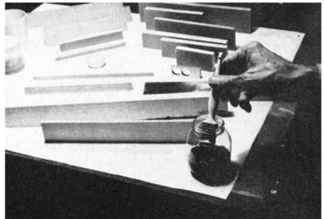
The job is now done and you have a variety of sanding blocks. Remember to clean the brush for next time. We used Bestine to clean out cement
